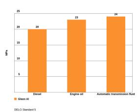
Elongation at tear after temperature storage, by the criteria of DIN EN ISO 527
