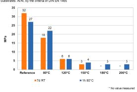
Compression shear strength on different substrates, DELO Standard 5 curing: 1h +80°C
