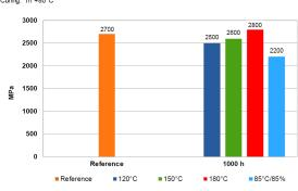
Young's Modulus after temperature storage, by the criteria of DIN EN ISO 527 Curing: 1h +80  $^\circ\text{C}$
