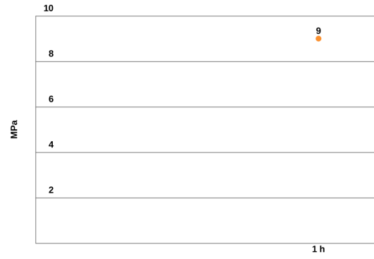
Tensile shear strength for determining the curing process at temperature Substrates: Al/Al, curing: 80 °C, by the criteria of DIN EN 1465
