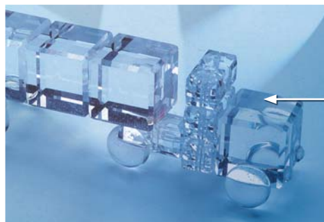
Bonding of small areas of glass gemstones
