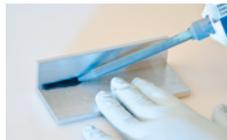
After work finish or during breaks, the mixing tube can usually remain on the cartridge as closure instead of the original closure cap.
