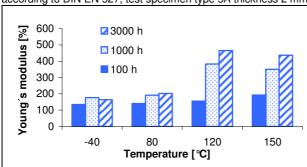
tensile strength after temperature storage based on initial value at room temperature measured at room temperature (approx. 23 ℃) according to DIN EN 527, test specimen type 5A, thickness 2 mm
